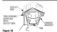
□ 2. Carefully lift the fan and seat the hanger ball/downrod assembly on the  $\Box$  1. Connect the green grounding lead from hanger bracket that was just attached to the outlet box (Figure 11). Be sure the groove in the ball is lined up with the tab on the hanger bracket (Figure 10).
